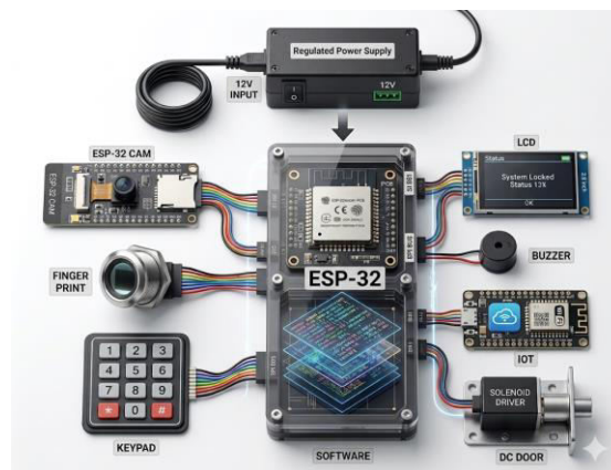
Figure 1. Block Diagram of Proposed Security System.
